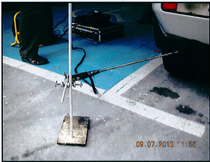
Figure 2 : Exhaust Emission Testing using Testo Gas Analyser
